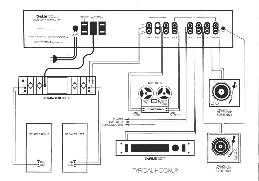
If the speakers are identical, then the resulting impedance is one-half of each speaker's impedance. (For example, two 8-Ohm speakers result in 4 Ohms when connected in parallel.)
