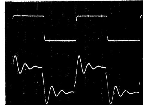
Fig. 7—10-kHz square waves; upper trace, low power into ohms (scale 5 V/cm, 20  $\mu$ S/cm); lower trace, low power into 2  $\mu$ F (scale 5 V/cm, 20  $\mu$ S/cm).
