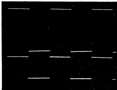
Fig. 6—50-Hz square waves; upper trace, 200 watts into 8 ohms (scale 20 V/cm, 5 mS/cm); lower trace, 3.12 watts into 8 ohms (scale 5 V/cm, 5 mS/cm).
