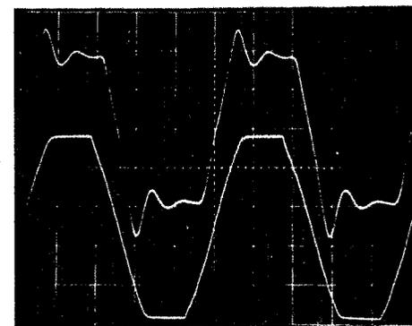
Fig. 9—Upper trace, 20-kHz, 80 V P-P square wave into 1  $\mu$ F load (scale 20 V/cm, 10  $\mu$ S/cm); lower trace, 20-kHz sine wave into 8 ohms with 2 dB overdrive (scale 50 V/cm, 10  $\mu$ S/cm).
