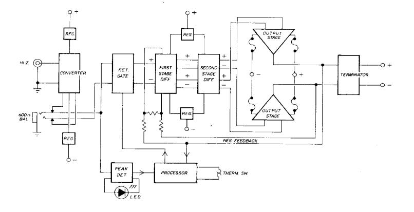
From the balanced input jack the signal goes to the FET gates. These gates are arranged as on-off switches in series and shunt and are activated by the protective processor in order to protect the amplifier against non-allowable states. Under normal operating conditions the gates are fully on and have been carefully designed in order to add no degradation to the audio signal. The distortion of the gates is at least an order magnitude below that of the main amplifier.
