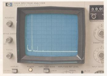
ACTUAL PHOTOGRAPH of harmonic distortion measurement, as measured by a Hewlett-Packard 3580A Spectrum Analyzer, through the phono and aux sections of an Infinity FET Preamplifier chosen at random from the shipping dock.
